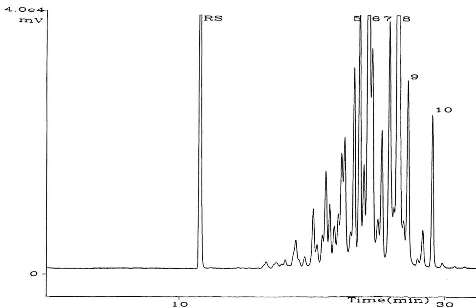
Fig. 2. HPLC of a human milk sample which was rapidly heated at  $80^{\circ}\text{C}$ , held at this temperature for 1.5 min, and then stored at  $-20^{\circ}\text{C}$  for 4 months. Peaks identified in Fig. 1.
