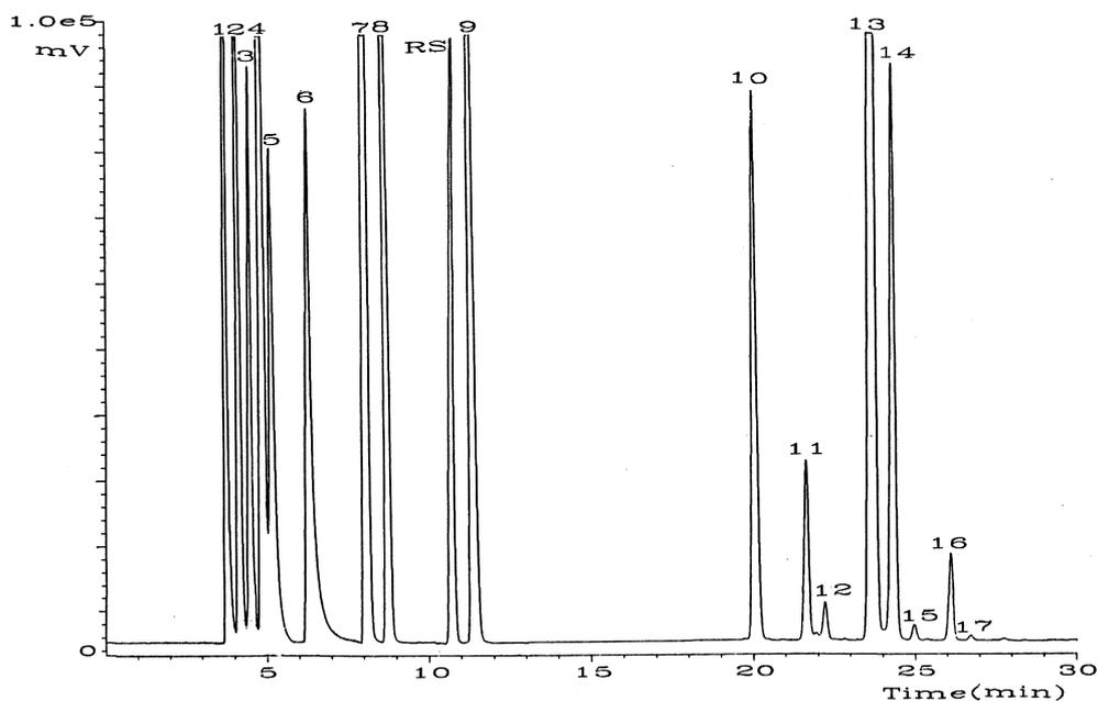
Fig. 6. Chromatogram of standard mixtures. Peak identification (for abbreviations see Table 1): (1) 1-monomyristoyl glyceride, (2) linoleic acid, (3) 2-monopalmitoyl glyceride, (4) oleic acid, (5) palmitic acid, (6) stearic acid, (7) 1,3-dimyristoyl glyceride, (8) 1,2-dimyristoyl glyceride, (9) 1,3-dipalmitoyl glyceride, (10) MMM, (11) LOO, (12) OPL, (13) OOO, (14) OPO, (15) PPO, (16) SOP.
